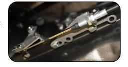
Ensure any gear safety mechanism is disconnected inside the steering column. This may stop the vehicle selecting the crank position while the vehicle is not in the park
