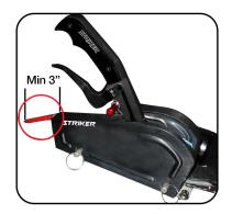
Note: make sure the shifter has clearance to dashboard and seats when moving through all the gears. Check this prior to drilling holes or mounting shifter
