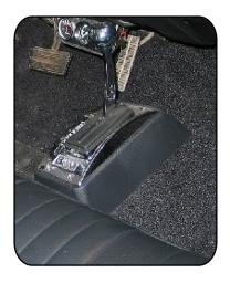
Note: make sure the shifter has clearance to dashboard and seats when moving through all the gears. Check this prior to drilling holes or mounting shifter
