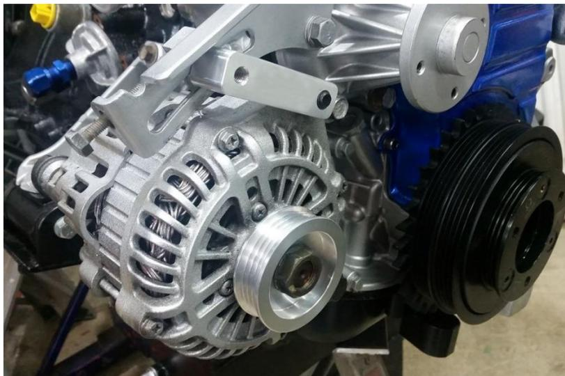
*Figure 1: Photo of GM Alternator mounted to RB Engine*
