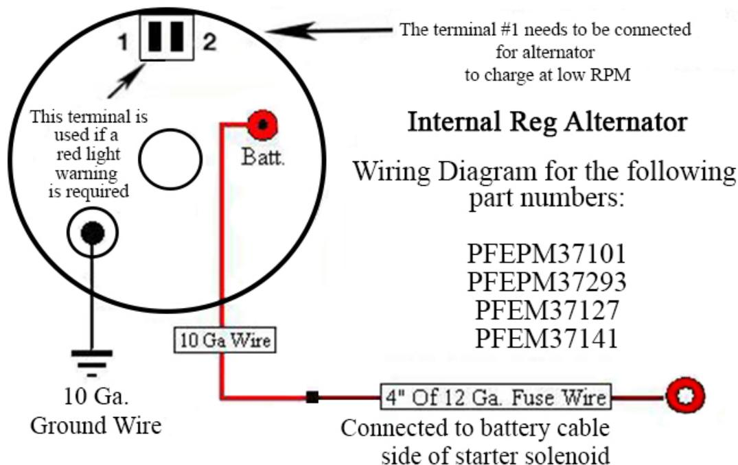
**GROUNDING REQUIREMENTS:** In order for an alternator to charge properly, the alternator must be grounded to the engine block. If an alternator has paint or clear-coat on the mounting surfaces, it may not be grounded and will not charge.
