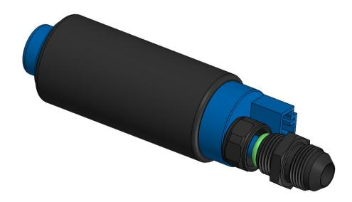
**NOTE:** Do not overtighten the nut as only a snug fit is required for sealing. Overtightening can damage the barb and/or o-ring. A gap may also be present between the nut and the bottom of the hex of the fitting which is normal. Gap size may vary depending on variations in barb designs.
