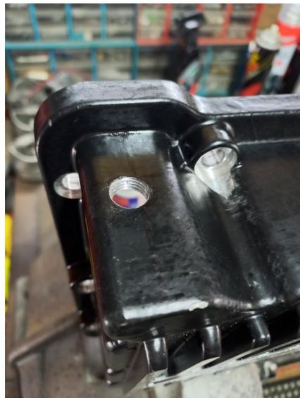
3. Temporarily screw both fittings into pan, hold pan up against transmission and mark the angle you need for the npt fitting to be at the best angle for hose to be snug against gearbox casing. You now need to put thread sealer on fitting and lock this into needed position while on the workbench as this needs to be fitted prior to mounting pan. You can now fit your pan using a new gasket and are ready to assemble the dipstick.
