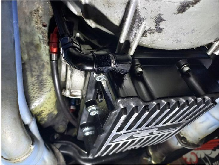
7. Gradually fill transmission with oil, starting vehicle between filling to bleed oil circuit. Get vehicle up to running temperature. Set to full mark and check for leaks.
