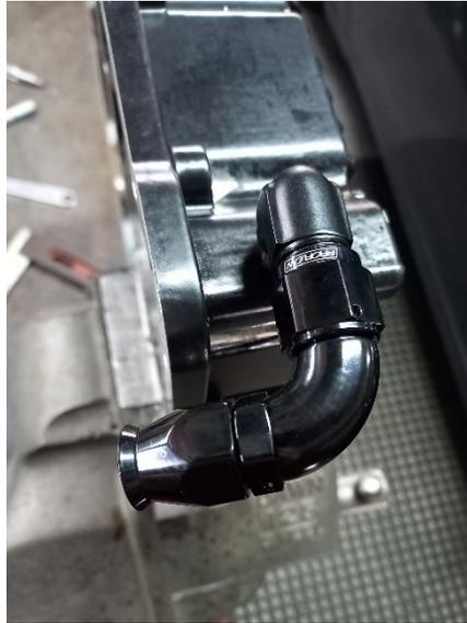
4. Decide where you will mount the supplied firewall dipstick tube mounting bracket, or fabricate your own bracket to mount on head/block etc. Once the tube has been mounted in a convenient position, screw your 200 Series elbow back onto pan and mark outer hose against pan fitting. Remove hose and elbow to cut hose to needed length and assemble hose end. Wash and blow out hose to be clean and ready for use. Now is a good time to calculate dipstick length to read correct fluid level.
