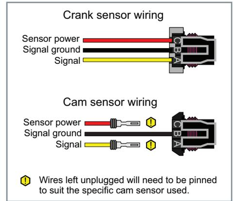
CAM SENSOR PLUG PINOUT WIRING
