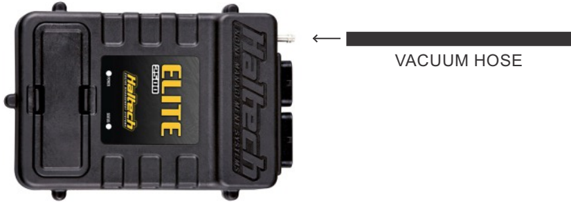
Figure 3 - Elite ECU internal MAP sensor
