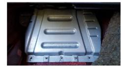
Figure 2 - Factory protective plate covering Haltech products
