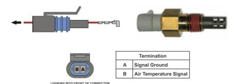
INSERT WIRE THROUGH PLUG, THEN CRIMP THE PIN INTO THE WIRE AND DRAW BACK TO LOCK
