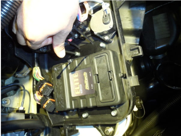
Figure 5 – Mounting Elite ECU to PWC
