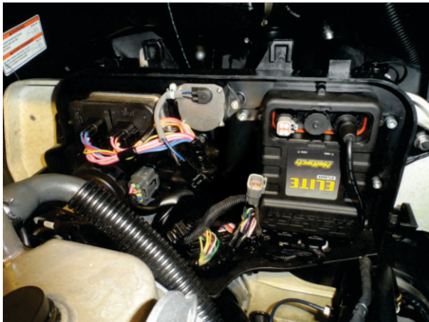
Figure 8 – Plug and Play Harness Installed
