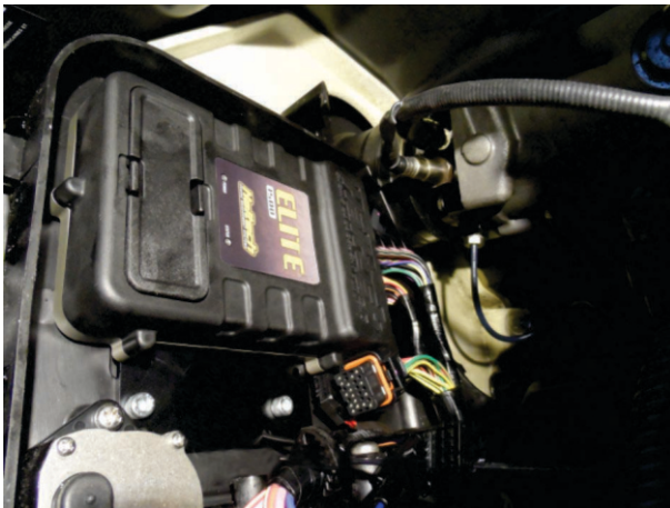
Figure 6 – Elite ECU Mounted in the OEM location.
