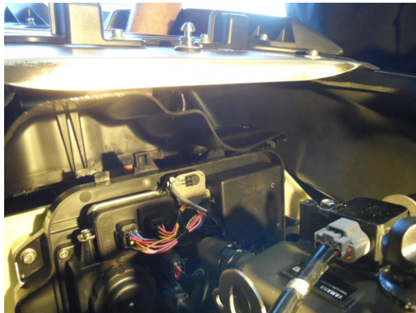
Figure 4 – OEM ECU Mounted on support
