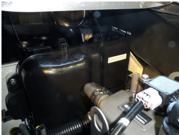
Figure 10 – Splash cover re-installed
