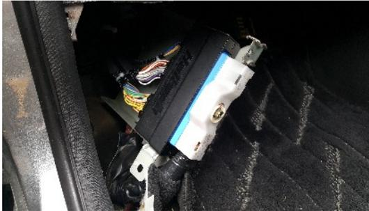
Figure 3 - Typical Plug 'N' Play Adaptor installation
