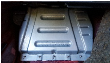
Figure 2 - Factory protective plate covering Haltech products
