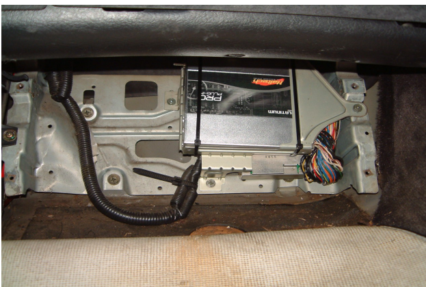
Figure 4 – Platinum Pro Plug-in ECU mounted in factory location
