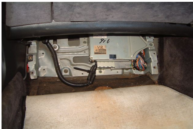
Figure 2 – Factory ECU Mounting Location with cover removed
