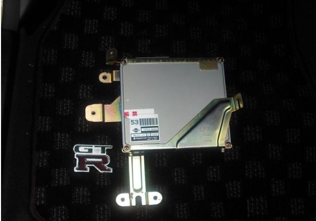
Figure 2 – Factory ECU disconnected and removed
