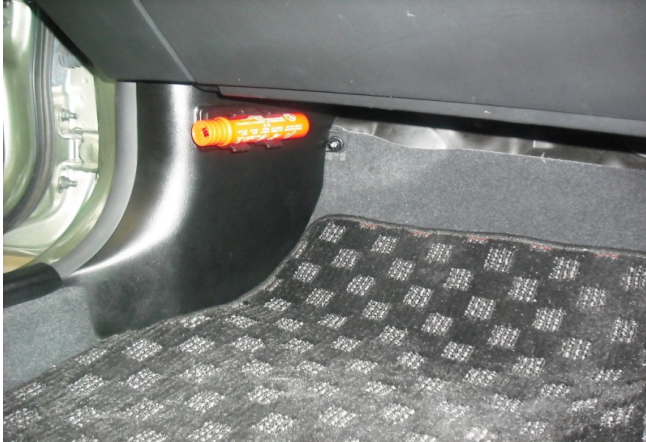
Figure 6 – Kick panel Re-installed
