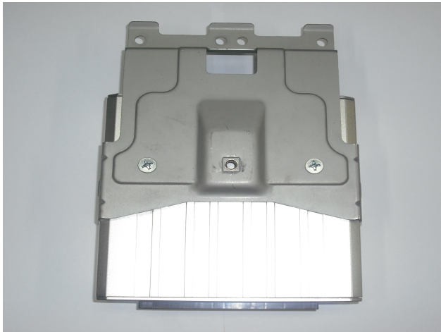
Figure 5 – Haltech ECU with original mounting bracket fitted
