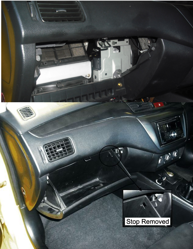
Figure 3 – Factory ECU Location (Glove Compartment Removed)
