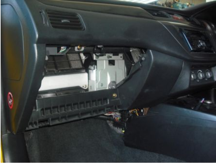
Figure 6 – Haltech Pro Plug-in ECU Installed
