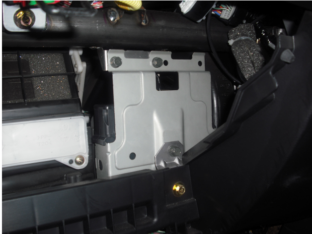
Figure 4 – OEM ECU in Original Mounting Position
