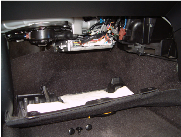
Figure 2 – Factory ECU location with cover removed
