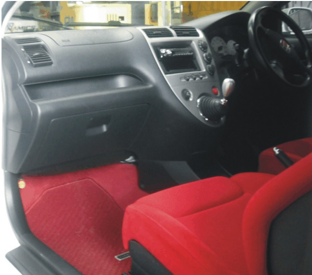
Figure 6 – Glove compartment and lower cover Re-installed
