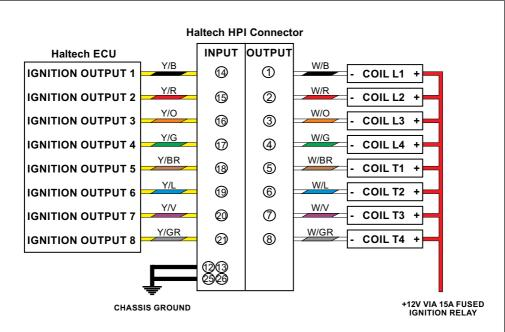
Figure 11 – 4 Rotor Direct Fire
