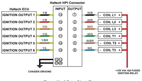
Figure 10 – 3 Rotor Direct Fire
